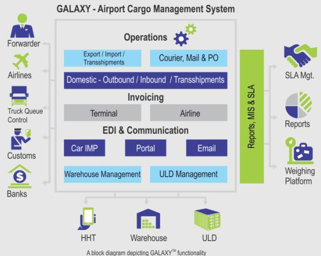
GALAXY™ GHA is a state-of-the-art ground handling module that supports the airports handling cargo in controlling the movement and storage of cargo at the warehouses and managing the transactions. It automates the operational processes and provides comprehensive information on consignment status, cargo tracking and terminal operations to all stakeholders.
